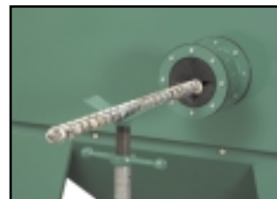
Specialized port allows easy cleaning of feed screws.
