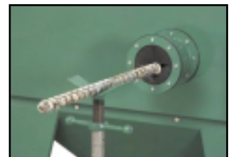
Specialized port allows easy cleaning of feed screws.
